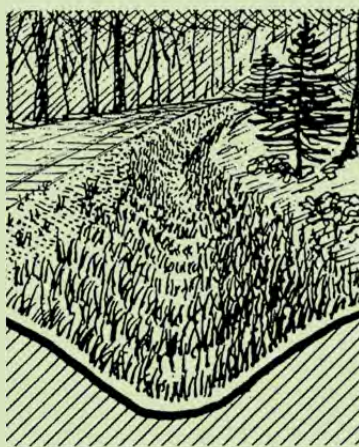
U-shaped, grass stabilized ditch
