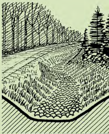
Grass and stone stabilized ditch
